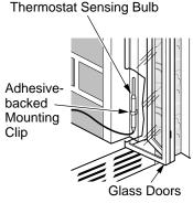
Figure 45-Installing Thermostat Sensing Bulb behind Glass Doors
